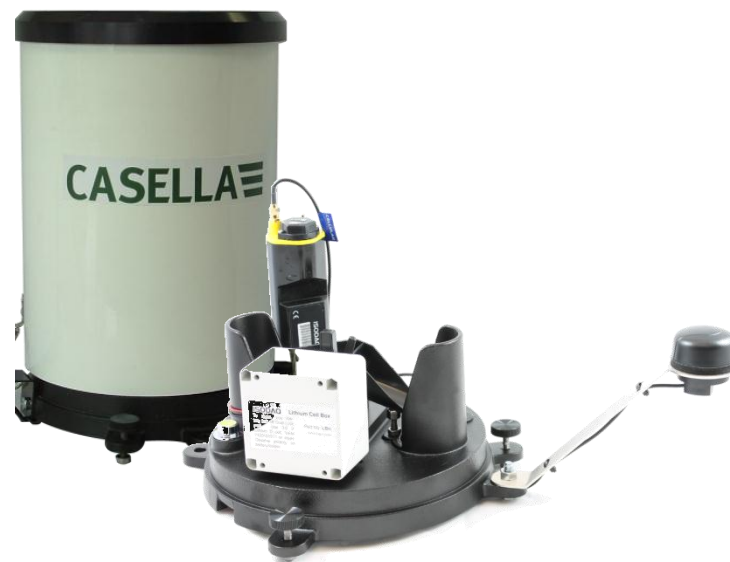
The STORM Guardian with the outer cover removed.
